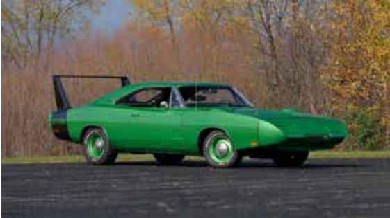
degrees versus the standard Charger's 45-degree backlight. The design had carried over from the Charger 500 along with A-pillar covers that smoothed the air flowing over the sides of the windshield and down the sides of the cars. On the Charger 500s and Daytonas, workers at Creative Industries carefully finished the bodywork around the plugs and repainted the roofs.
