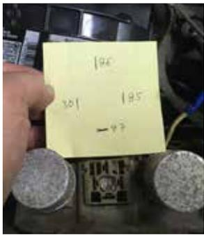
Terminal 30 on the relay socket has to be hot. I checked it with the multimeter, and it was. Since all that a relay does is connect 30 to 87, you can do that yourself with a jumper wire. This is often referred to as "bypassing the relay,"
