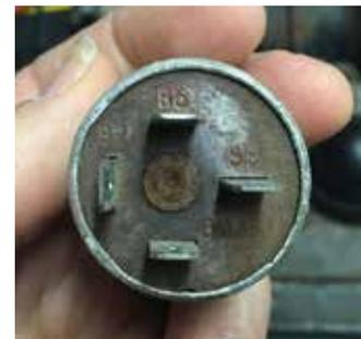
Next was the relay. In this car, there are three identical relays sitting next to each other (high beam, low beam, and horn). I swapped the
