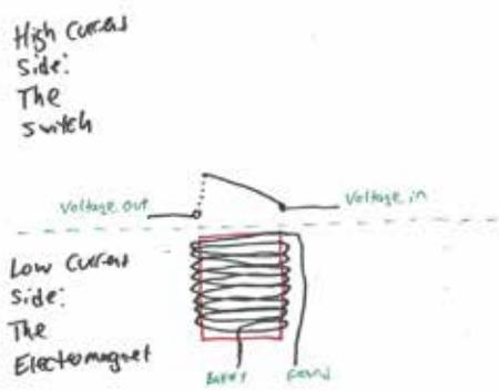
which pulls the relay's internal contacts together. That connects 30 to 87, allowing 12V to flow to the fan motor. Since the other leg of the fan motor is grounded, that turns on the fan. While there are other, more complicated relays that turn on one device while they switch another one off, this example contains 95 percent of what you need to know about relays. They are simple, elegant, and actually quite beautiful things.
